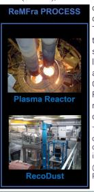
carbon smelting reduction process developed by Tata Steel Nederland Technology). Further by-products to be tested in the Plasma Reactor part are secondary metallurgical slag from the ladle furnace (steel refining aggregate) and scale from the slab rolling mill. Current activities focus on the detailed ReMFra process design and the preparation of first melting and reduction campaigns.
